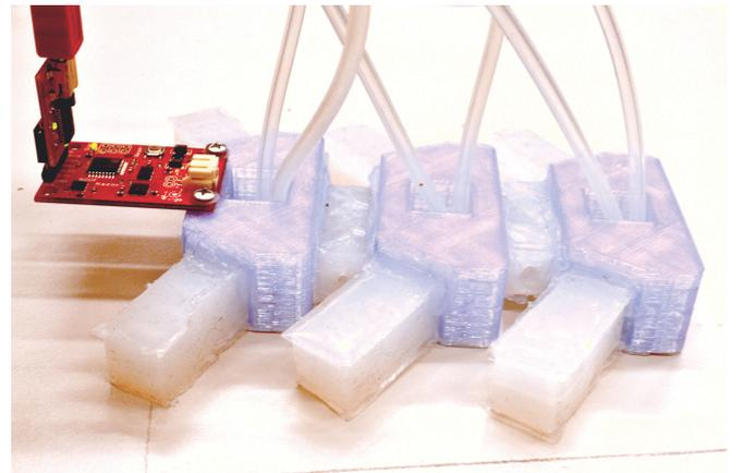
Fig. 5. Photo of the Robot with the Razor IMU attached at the rear end.
