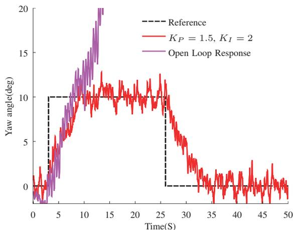
Fig. 11. Closed loop yaw angle response with a Proportional Integral controller. The open-loop response is drawn in magenta for comparison purposes.
