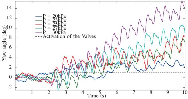
Fig. 9. Drift of the robot's yaw angle when identical pressure are applied to the front actuators. Here the robot advances without the walls, only by means of the friction between the actuator and the floor.
