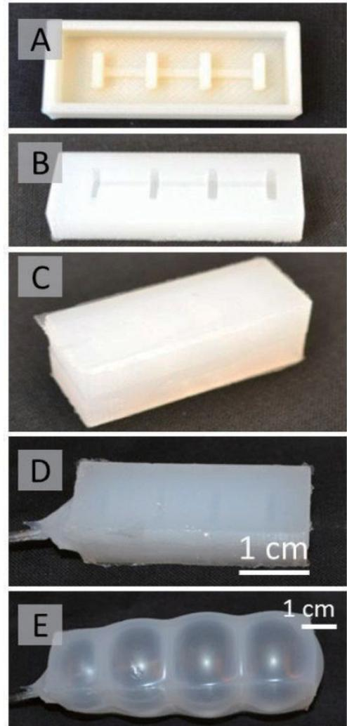
Fig. 2. The procedure of fabrication of a 4 chamber linear SPA. (A: the molds for making the linear SPA; B: the cured silicon rubber (half of actuator); C: The two halves bonded together with silicon glue; D: finished linear Actuator; E: Inflated Linear Soft Pneumatic Actuator.)
