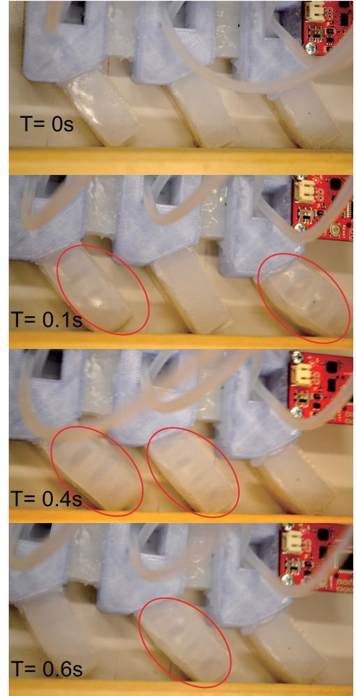
Fig. 8. Snapshots of the inflation pattern for one gait cycle (20 kPa, cycle period 1s) The red circle represents the actuator that is inflating at the time.
