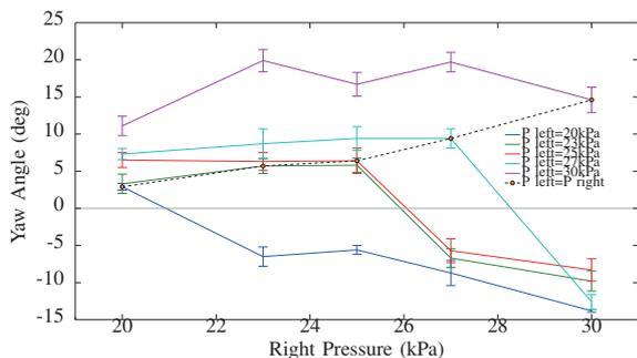
Fig. 10. Pressure combinations to achieve deviation (yaw angle). The black dotted line shows open loop drift when  $P_{\text{left}}$  and  $P_{\text{right}}$  are equal.
