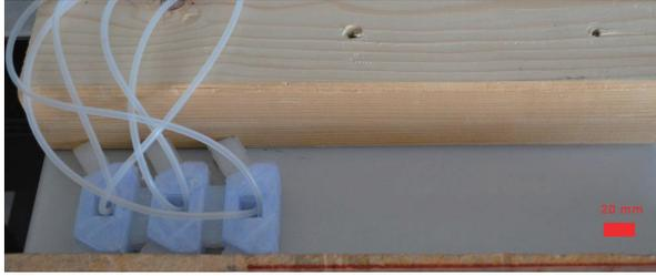
Fig. 6. The set-up used for evaluation of the propulsion capacity of the robot. The passage is 110 mm wide.
