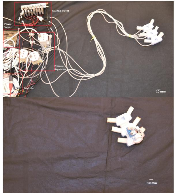
Fig. 12. Up: Current set-up including the robot’s and pneumatic system (pumps, servo valves, pneumatic driver and power source). Down: Untethered version. For clarity only one module has the pump embedded.
