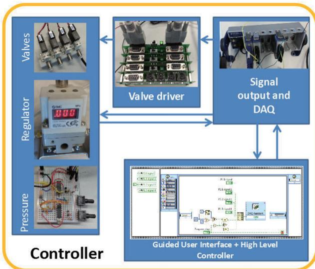
Fig. 4. Schematic of the pneumatic system
