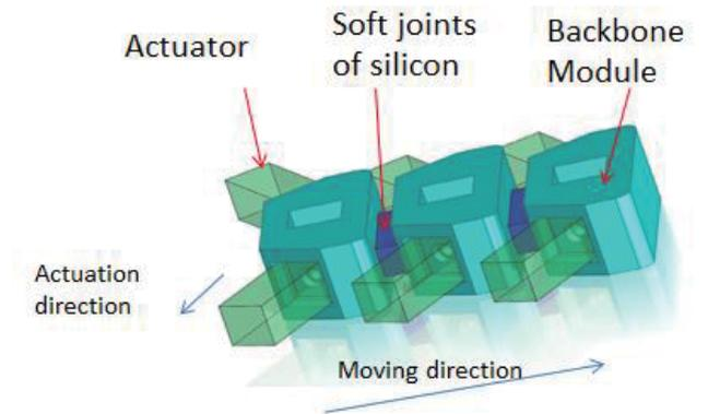
Fig. 3. CAD model of the robot
