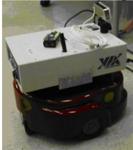
Charger, plugged into the robot computer
