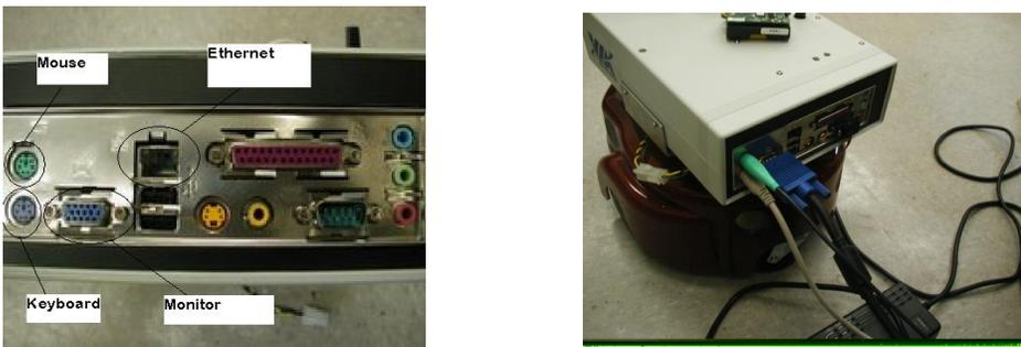
3. Make sure the robot is connected to the robot computer.
