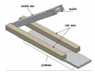
The Nail-It consists of three main components: the swinging arm with the mallet, the platform acting as a nail holder, and the sliding mechanism of the two side arms. The mallet is able to swing up and down because of the copper dowel that goes through the pivoting end of the arm and the two supporting sides.
